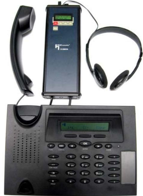
*H-QMON connected to IP phone, handset and headphone*
