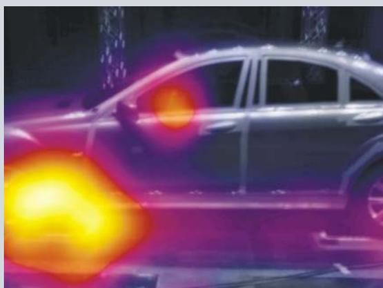
Shifting of the sound source indication in the wind tunnel
