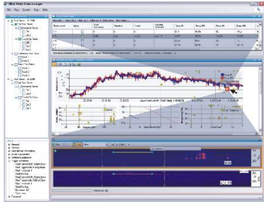
Figure 12: The results of large series of measurements can be managed with ease (tree and detailed views left). Selecting a series of measurements from the tree produces a tabular overview of the noise events along with their environmental conditions (above). There is also a complete report containing various freely-definable diagrams which display the noise events in correlation to their environmental conditions (middle). If you select a result from the table or a diagram, then the associated noise is played back on request and you can closely examine a spectral analysis of the event. You can interactively select different parameters for the X and Y axes (e.g. pressure, temperature, velocity). These parameters can be instantly correlated with the noise.
